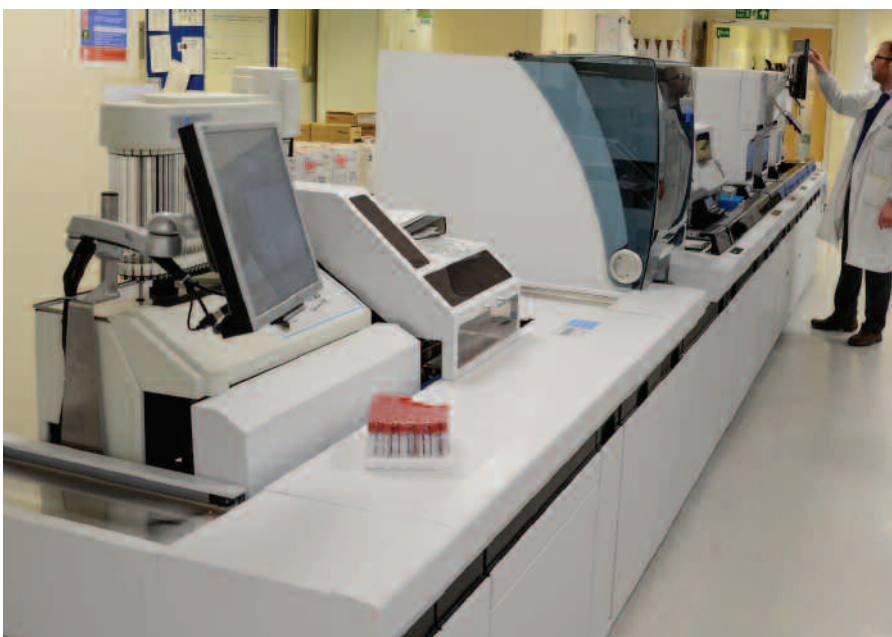
The XN series solution is a scalable and flexible combination of fluorescence flow cytometric haematology analysers, automated slide preparation and stainer, fully-automated ESR system and tube sorter.
